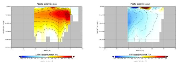
Note that autoscaling has been turned off and the min and max plotting limits set manually. By convention, streamfunctions are plotted with their scale symmetrical around zero, giving red and 'warm' colors for positive value and clockwise overturning, and blues and 'cold' colors for negative values and anti-clockwise overturning. Also shown is the same for the Pacific. (The plots have been tart-ed up by overlaying solid contours plus contour labels.)
